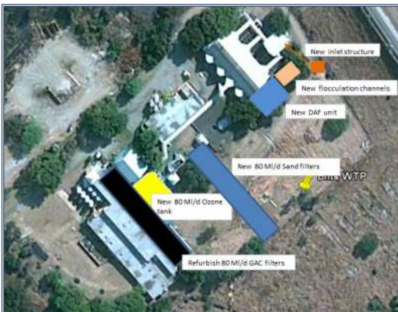
Several aspects had to be taken into account with the process design such as the possibility of the quality in the Hartbeespoortdam to improve and the option of laying a raw water pipe or utilizing the existing canal to convey the raw water to the new plant.
